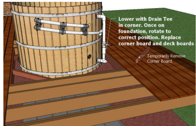
Figure 16 - Lowering Tub through the Opening
