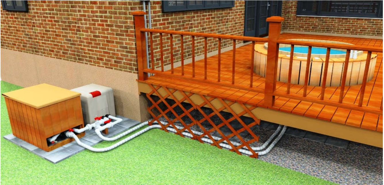
Figure 28 -Remote Location of Equipment pad and Gas Heater
